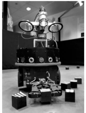
Robot Darwin VII - mobile base equipped with several sensors and effectors and a neural simulation running on a remote computer workstation
