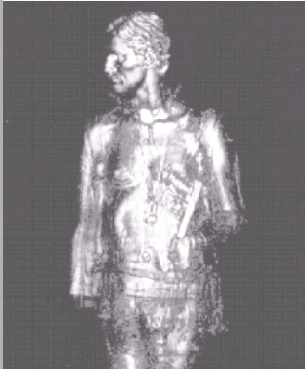
Holographic image of subject in millimeter-wave portal develop by Battelle Northwest National Laboratory. Array operating in the Ku band (10-20GHz).
