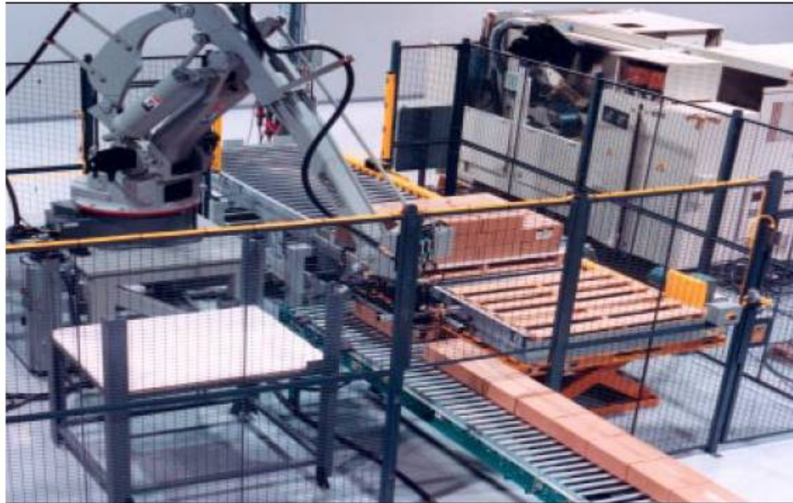
Motoman SP100 robot with vacuum gripper palletizes cases of filters.
